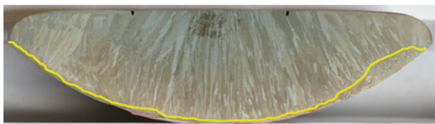
Fig. 4 Macrograph of a sectioned button of nickel-based superalloy
